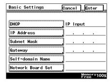
7 With the keypad in the operation panel, type in the IP address, and then touch [Enter].
